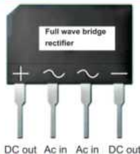
Figure 17.16(b): A Compact Full wave Bridge Rectifier used in electronics.
