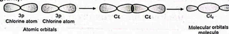
Figure: Overlap of p and p orbitals to form Cl 2 molecule according to VBT
