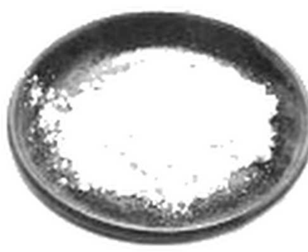
Figure 5.6: Heat is produced when quicklime is slaked
